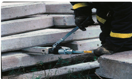
Hand operated spreader with 4.5 ton capacity.
